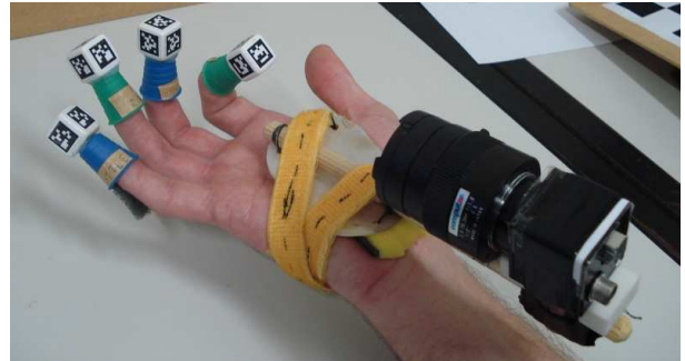
Figure 1. The Image-Based Data Glove prototype: a camera attached to the user's hand tracks his/her fingers using real-time computer vision techniques. Information about finger movements are estimated using inverse kinematics techniques.
